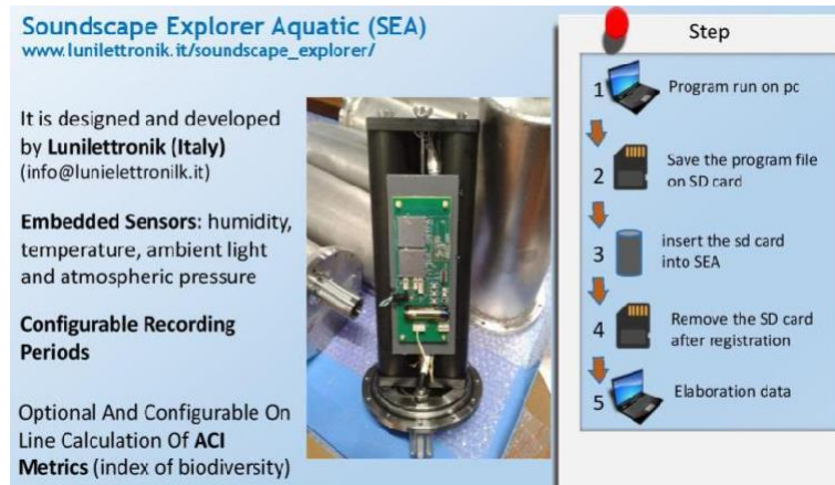
Figure 14. Hydrophone for measuring the sound pressure level in the area of interest.
