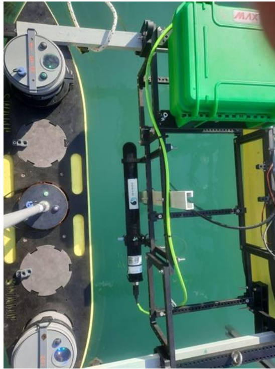
Figure 15: SUNA-V2 Installed on SWAMP.
