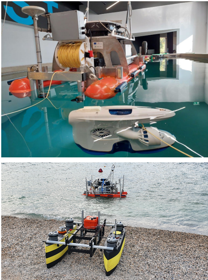
Fig. 1: Korkyra catamaran with tether management system and tethered Blueye ROV deployed in LABUST pool (above), SWAMP catamaran ready for deployment alongside Korkyra and Smart Buoy in Biograd na Moru, Croatia (below).
