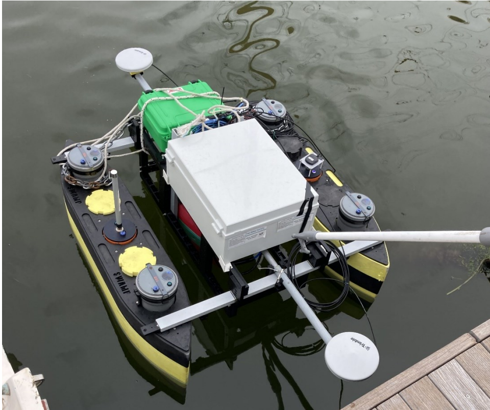
Fig. 3: R2Sonic MBES system integrated on SWAMP
