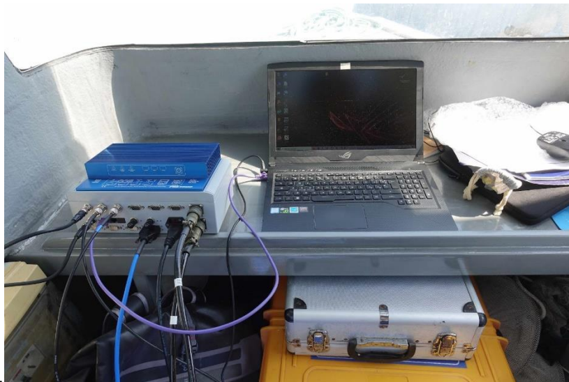
Figure 2: Working station mounting the acquisition software connected with SIM (on the right)
