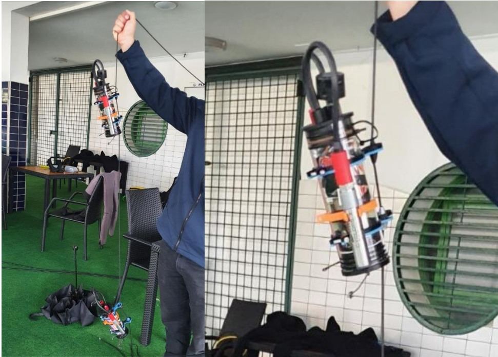
Figure 9. Sensor units attached to mooring line
