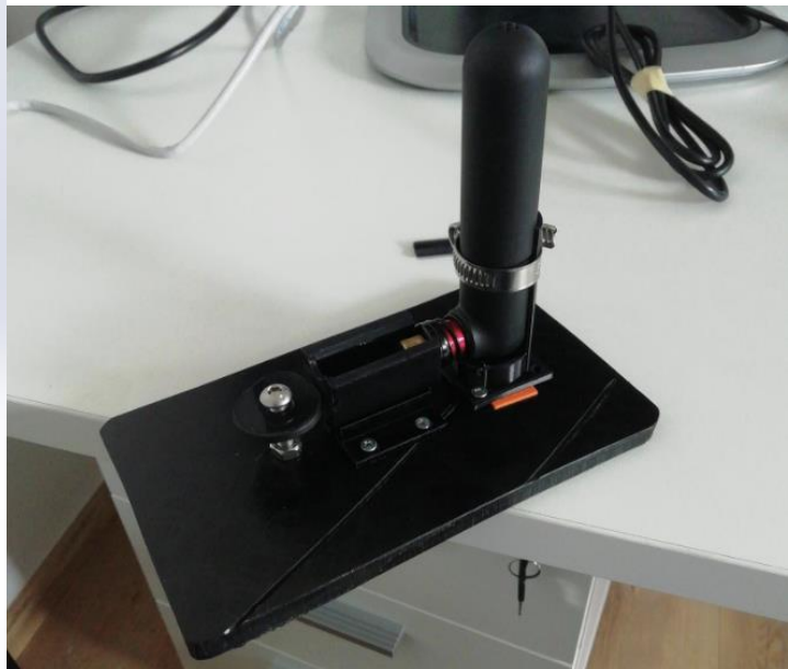
Fig. 18 First prototype for inflation mechanism (in 3D concept and the designed version).
