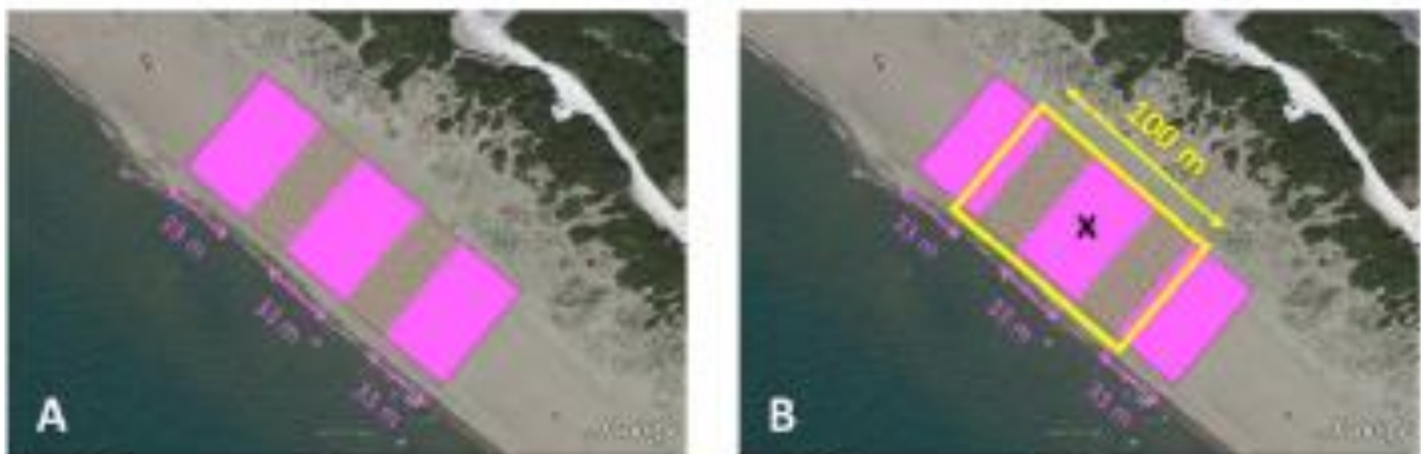
Fig. 1 – (A) Sampling up to 2019: three 33m areas (in pink). (B) New sampling (from 2020): single 100 m transect (in yellow). The centroid (black X) of the new transect closely matches the centroid of the three 33 m areas of the previous cycle of surveys.
