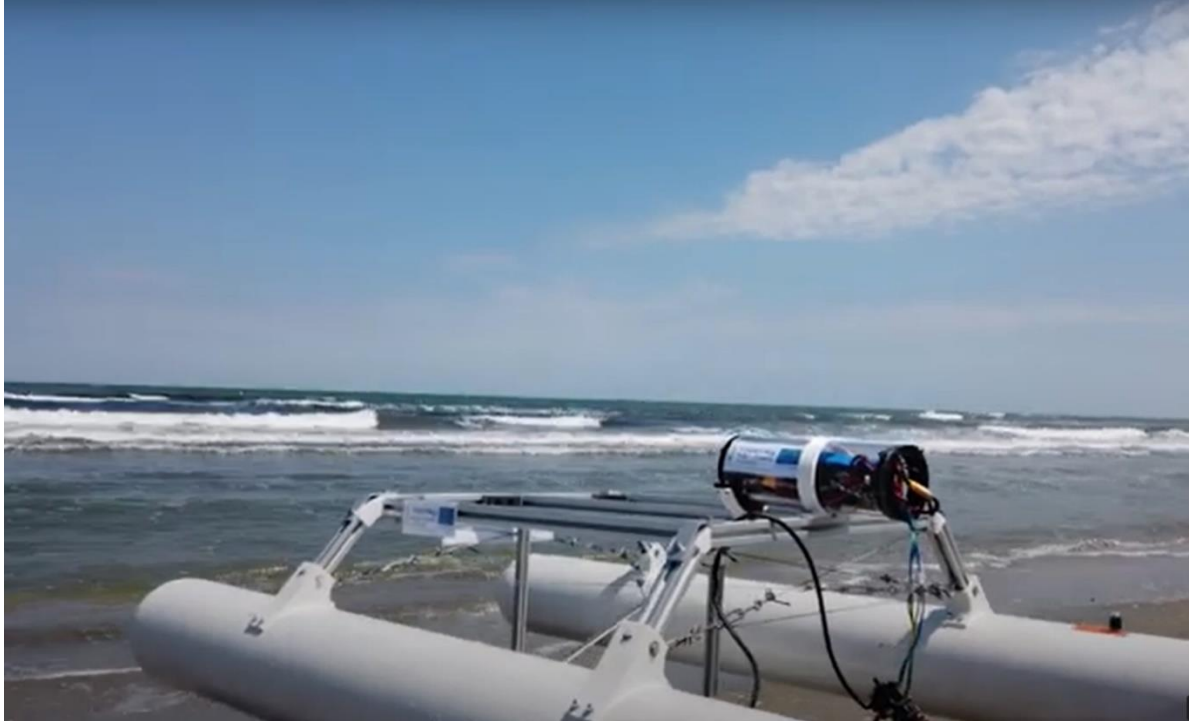
Figure 9. Water drone for plastic collection (PP6 – University of Bologna)
