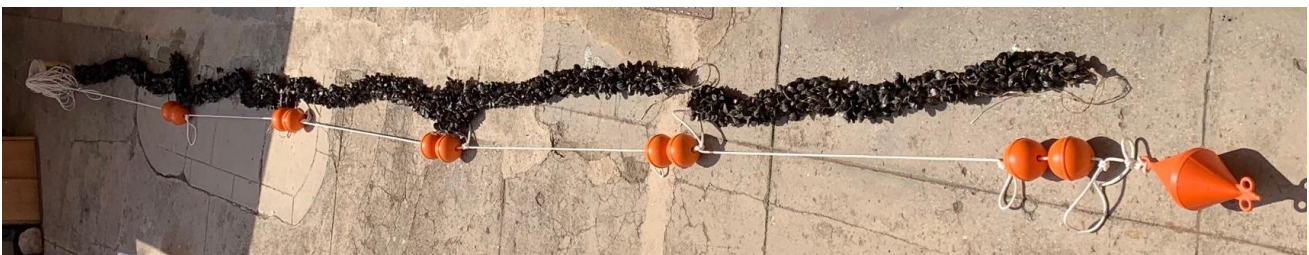
Figure 6.4.6. Mussel MicroPlastic Purification installation (MMP-P).
