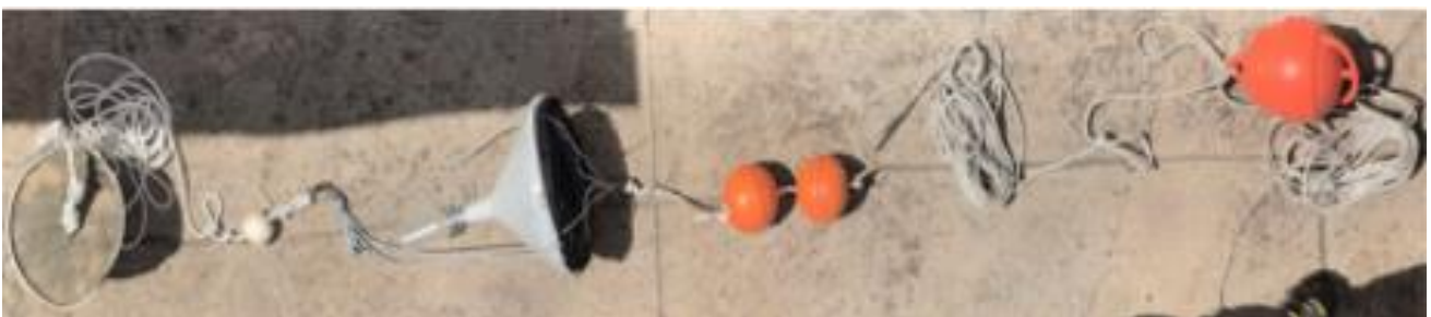
Figure 6.4.5. Mussel MicroPlastic Monitoring installation (MMP-M).
