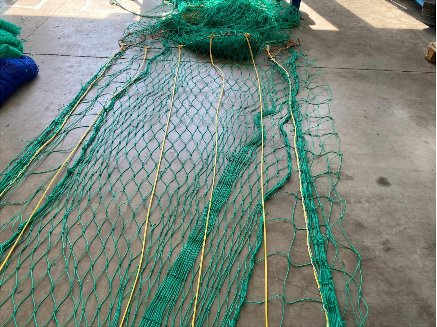
Figure 2 - Detail of the longitudinal ropes in the upper part of the net.
