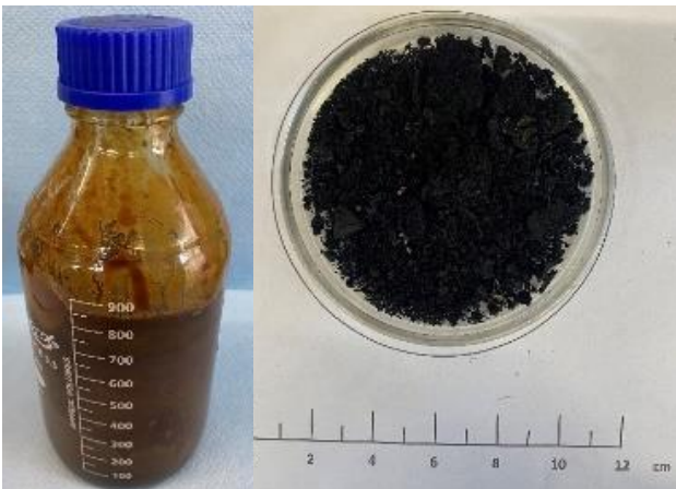
Figure 5.5 Oil and solid product of pyrolysis, © Fraunhofer UMSICHT
