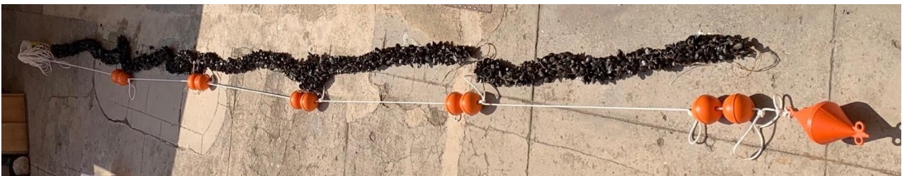
Figure 6.4.19. Mussel MicroPlastic Purification installation (MMP-P).
