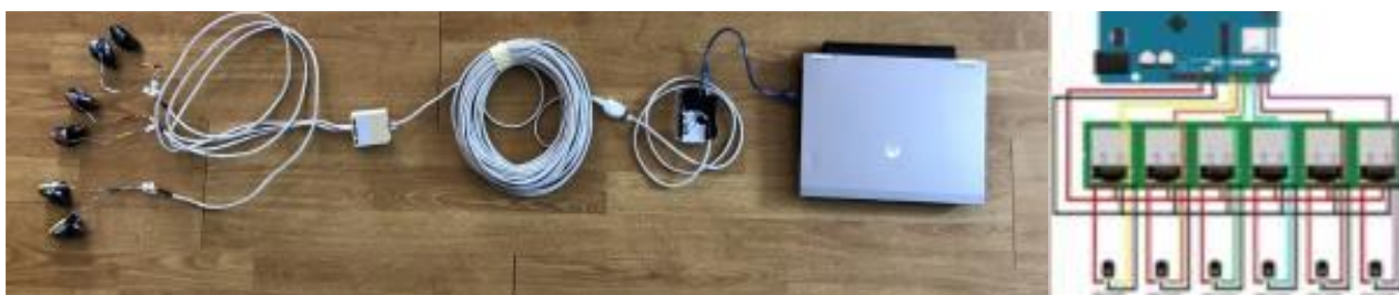
Figure 6.4.5. Valve Gaping Mussel Monitor (VGMM) with 6 sensors/mussels and Arduino microcontroller VG Hall sensors connection schema.
