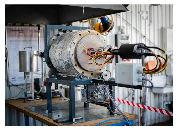
Figure 3.1.2 Batch-scale plant for the thermo-chemical conversion, © Fraunhofer UMSICHT
