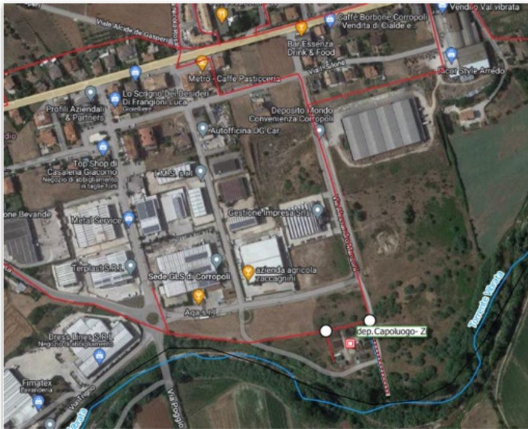
Figure 3 This image provides a visual representation of the Corropoli wastewater treatment plant and the two main sewer lines feeding into it. The two white dots are the combined sewer overflow stormwater overflow located at the end of these sewer lines. These CSOs play a crucial role in managing excess water during intense meteorological events.
