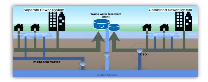
**Separate Sewer System**: it is a sewer system where domestic wastewater and stormwater are managed separately. There are two distinct pipe networks: one for domestic and industrial wastewater and another for stormwater runoff from street and
