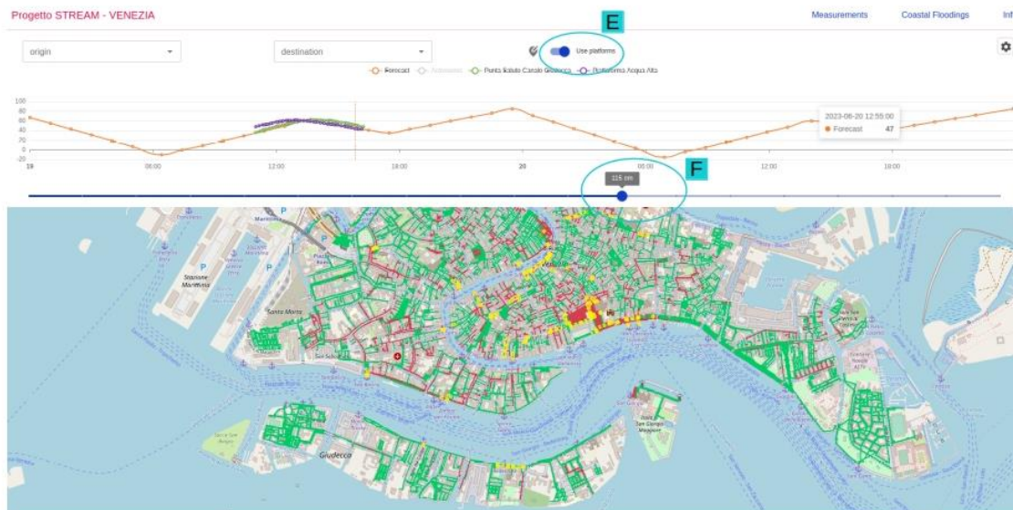
Fig. 3 HomePage: switch (E) to activate/deactivate usage of platforms during the routing calculation. Selection of specific height of sea level through the Slider (F).
