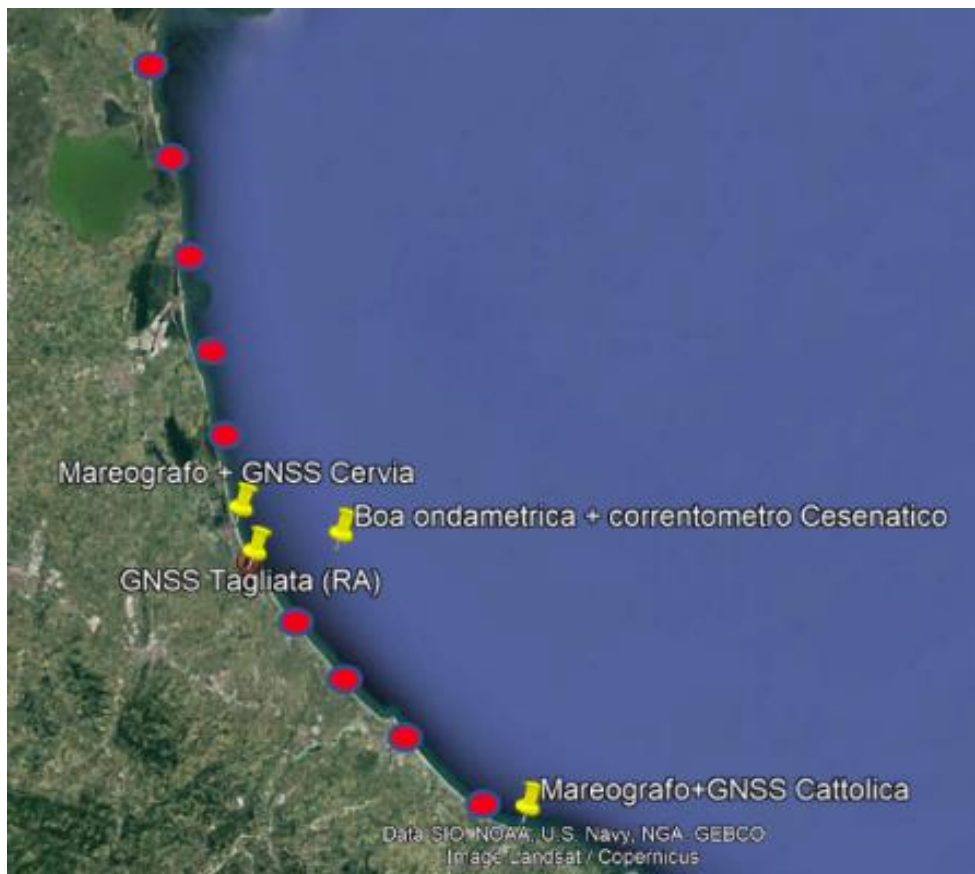
Figure 5. Location of the tide gauges installed along the Emilia-Romagna coast. In addition to that, other equipment (e.g. wave buoy - Boa ondamentrica + correntometro) purchased and installed recently are also shown.
