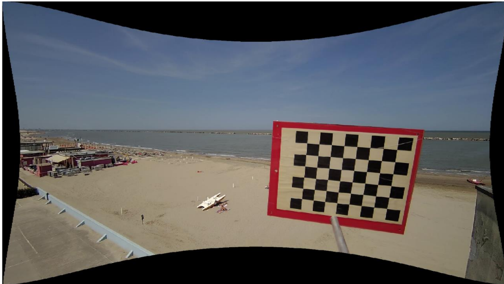
Annex A3. Corrected A1 image with rectified dimensions and all pixels being shown (the invalid pixels are filled in this image, contrary to what happens in image A2 in which the pixels are deleted from the image).
