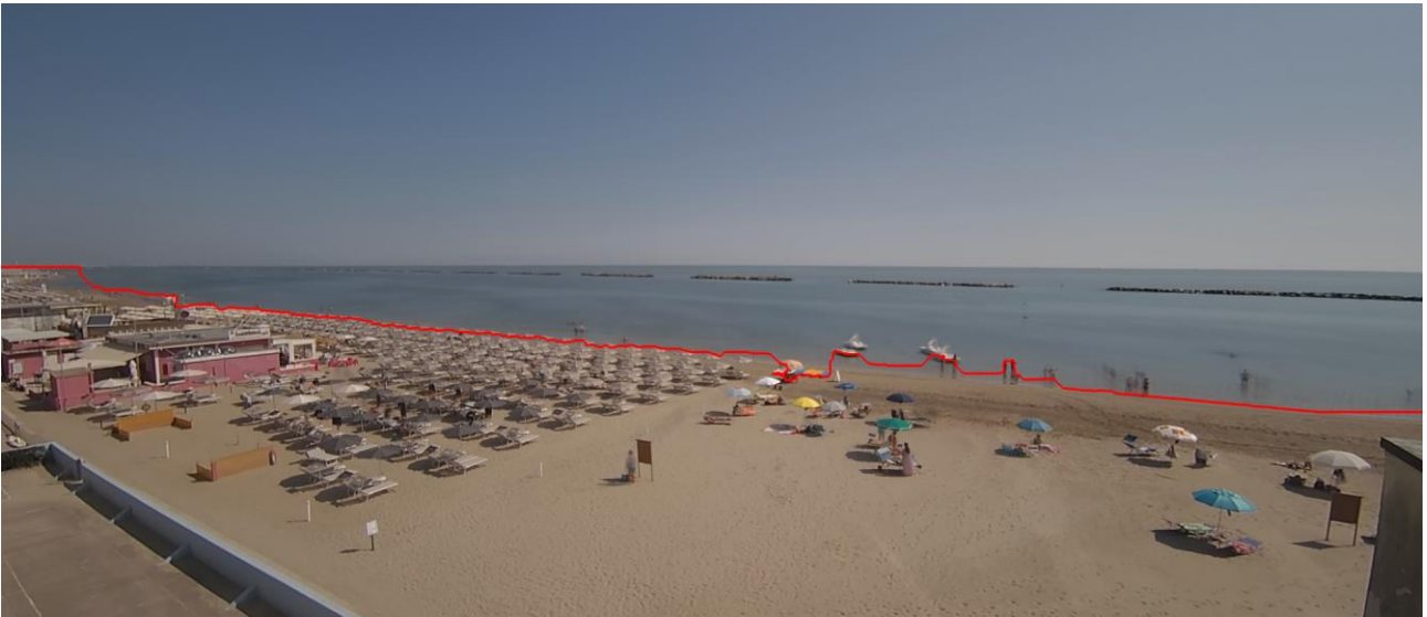
Annex A5. Timex (produced with 50 images) with the shoreline mapped (Valverde webcam)
