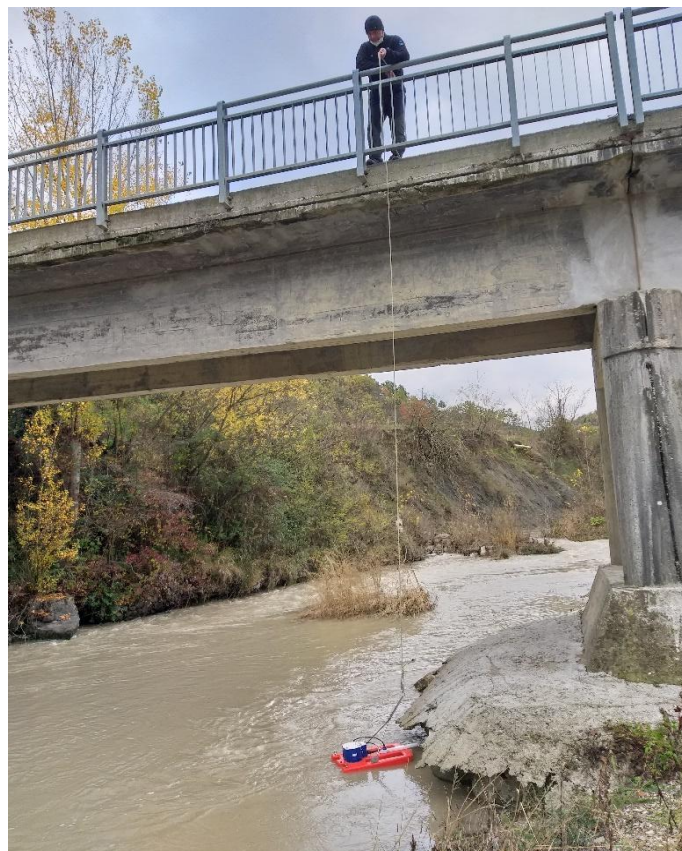
Fig. 1 Flow measurement at Mercatale station (Foglia basin)
