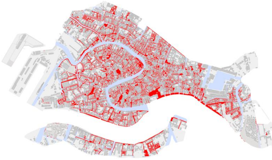
Figure 6: Flooding map of the city of Venice according to the predicted sea level height of 160 cm. Light blue colour indicates the canals.
