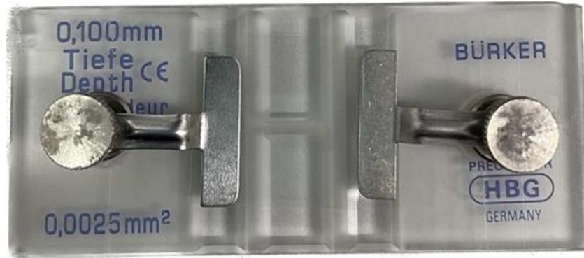
Figure 7: Bürker chamber for algal cell count.
