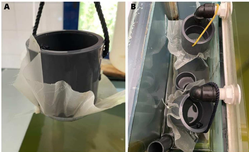
Figure 20: Collectors with mesh 120 \mu for the collection of veliger (160 \mu ).
