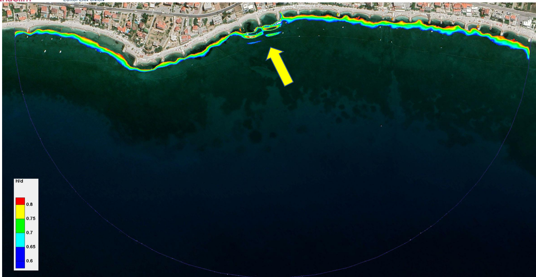
Figure 6.63 – Wave breaking zone for Simulation A25 – conceptual design for the control area (marked with a yellow arrow) of the beach on the Podstrana-Duče area with wave parameters from the Direction of SSW (202.5°), 50-year return period ( H_s=2.09 m; T_p=5.90 s) and sea level corresponding to absolute maximum
