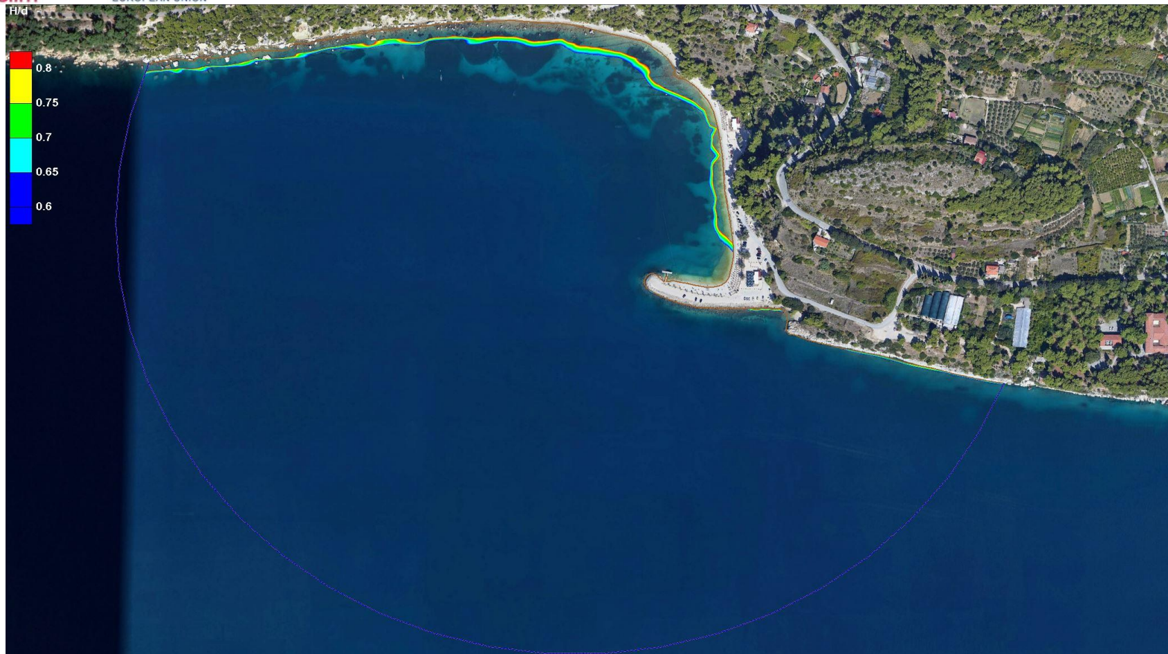
Figure 6.71 – Wave breaking zone for simulation A27 – the existing state of Kašjuni beach in Split with wave parameters from the Direction of SSW ( 202.5^\circ ), 50-year return period ( H_s=1.57 m; T_p=5.11 s) and sea level corresponding to middle sea level (SRM)
