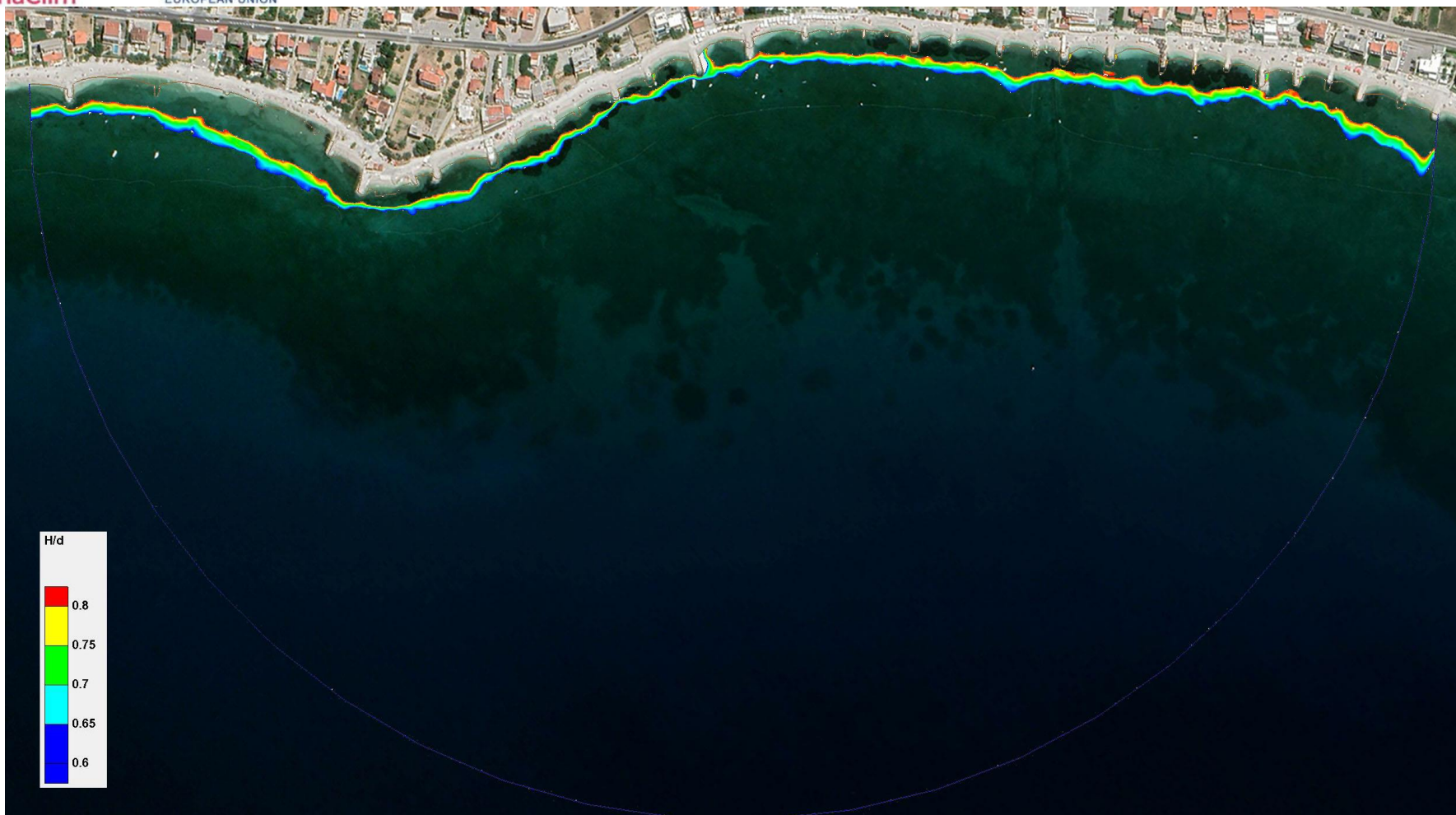
Figure 6.66 – Wave breaking zone for simulation A20 – the existing state of the beach on the Podstrana-Duče area with wave parameters from the direction W (270°), a 50-year return period ( H_s=1.73 m; T_p=5.36 s) and sea level corresponding to the middle sea level (SRM)
