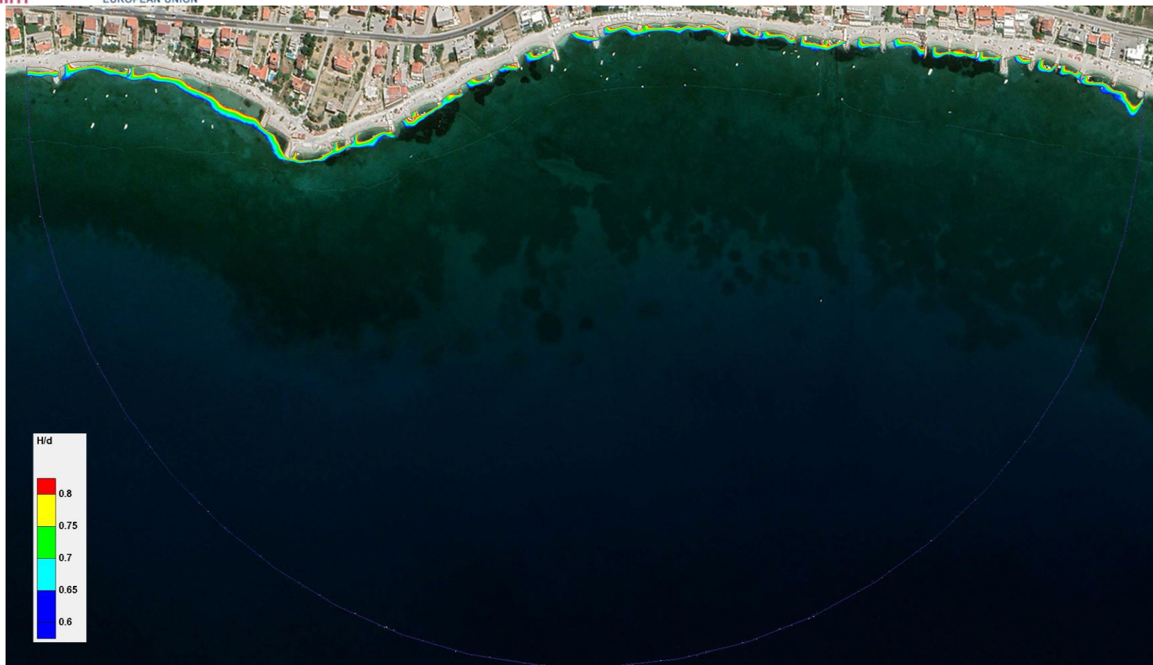
Figure 6.67 – Wave breaking zone for Simulation A23 – the existing state of the beach on the Podstrana-Duče area with wave parameters from the direction W (270°), a 50-year return period ( H_s=1.73 m; T_p=5.36 s) and a sea level corresponding to the absolute maximum
