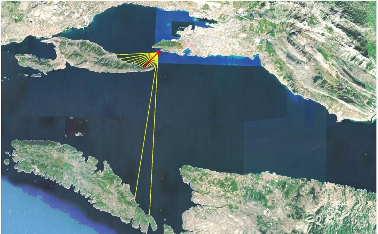
Figure 3.35 – Display of the central beam through the direction SW (225°), and the beam with step \pm 6^\circ
