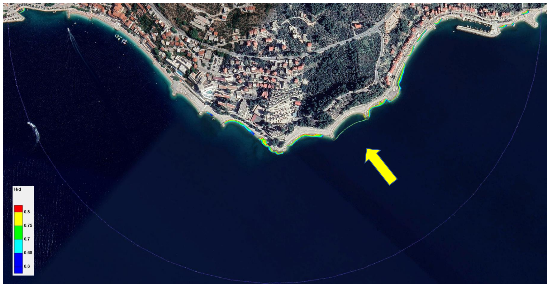
Figure 6.45 – Wave breaking zone for Simulation A17 – conceptual design for the control area (indicated by a yellow arrow) of Podgora beach (Makarska Riviera) with wave parameters from the Direction of SSE (157.5°), 50-year return period ( H_s=2.15 m; T_p=5.98 s) and sea level corresponding to absolute maximum
