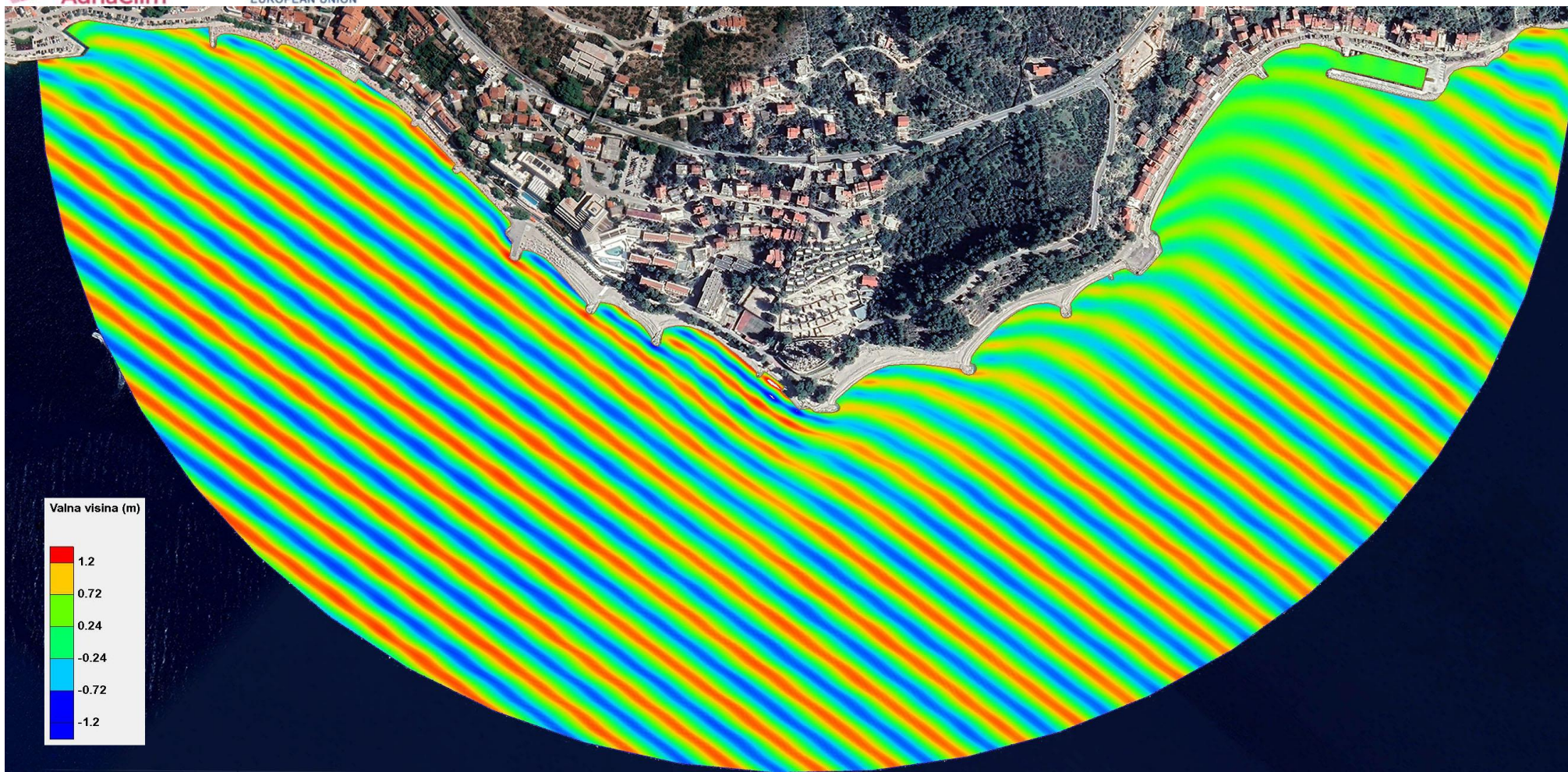
Figure 6.50 – Current wave outline for simulation A13 – existing state of Podgora beach (Makarska Riviera) with wave parameters from w direction (270°), 50-year return period ( H_s=2.32 m; T_p=6.21 s) and sea level corresponding to middle sea level (SRM)
