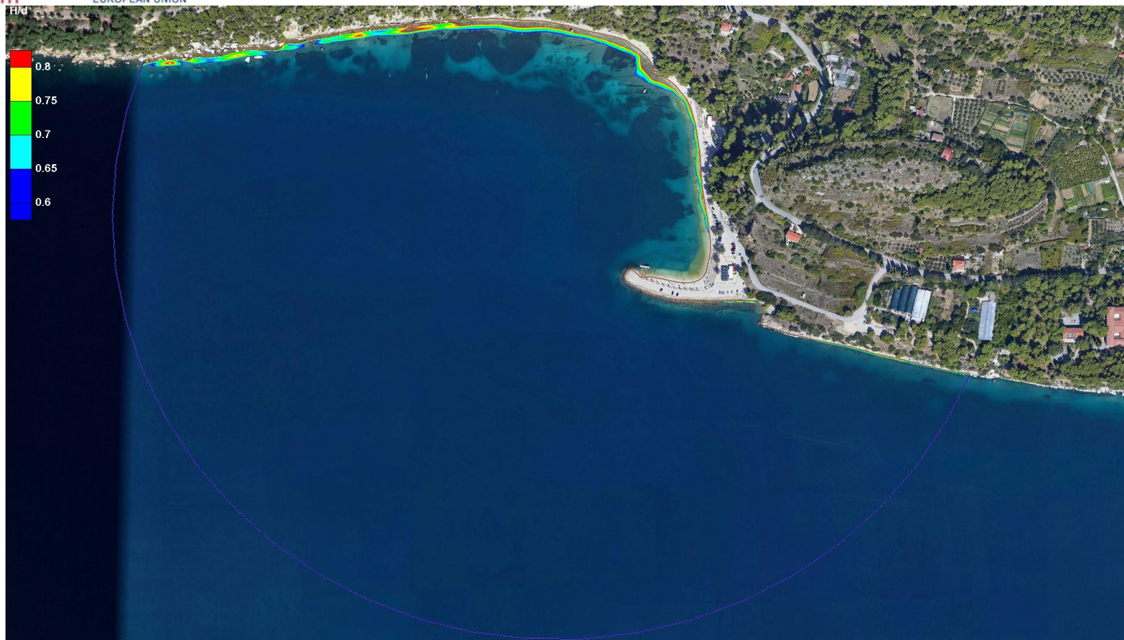
Figure 6.72 – Wave breaking zone for simulation A29 – the existing state of Kašjuni beach in Split with wave parameters from the Direction of SSW ( 202.5^\circ ), 50-year return period ( H_s=1.57 m; T_p=5.11 s) and sea level corresponding to absolute maximum
