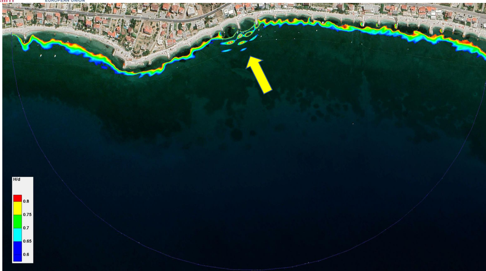
Figure 6.58 – Wave breaking zone for Simulation A24 – conceptual design for the control area (marked with a yellow arrow) for the beach on the Podstrana-Dučé area with wave parameters from the SE direction (135°), a 50-year return period ( H_s=2.46 m; T_p=6.40 s) and a sea level corresponding to the absolute maximum
