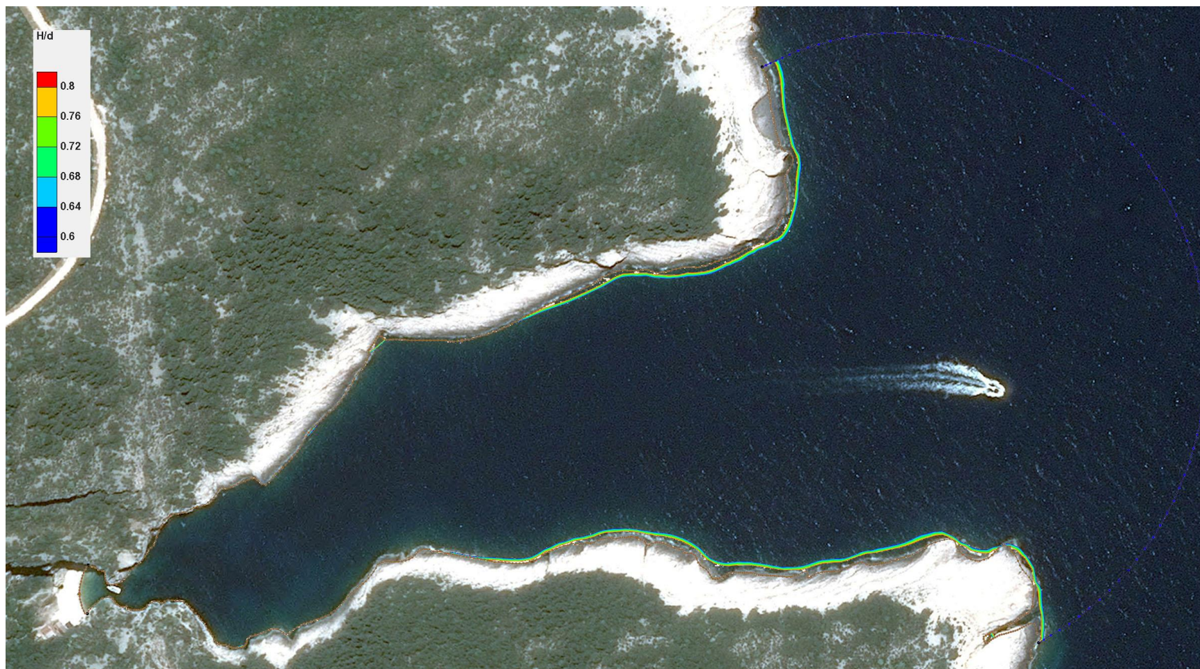
Figure 6.40 – Wave breaking zone for simulation A9 – existing state of Stiniva beach (Vis) with wave parameters from the direction of SE (135°), 50-year return period ( H_s=4.81 m; T_p=8.94 s) and sea level corresponding to middle sea level (SRM)
