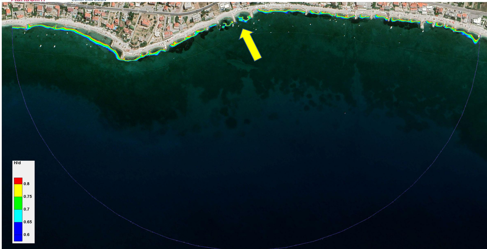
Figure 6.68 – Wave breaking zone for Simulation A26 – conceptual design for the control area (indicated by a yellow arrow) of the beach on the Podstrana-Duče area with wave parameters from w direction (270°), 50-year return period ( H_s=1.73 m; T_p=5.36 s) and sea level corresponding to absolute maximum
