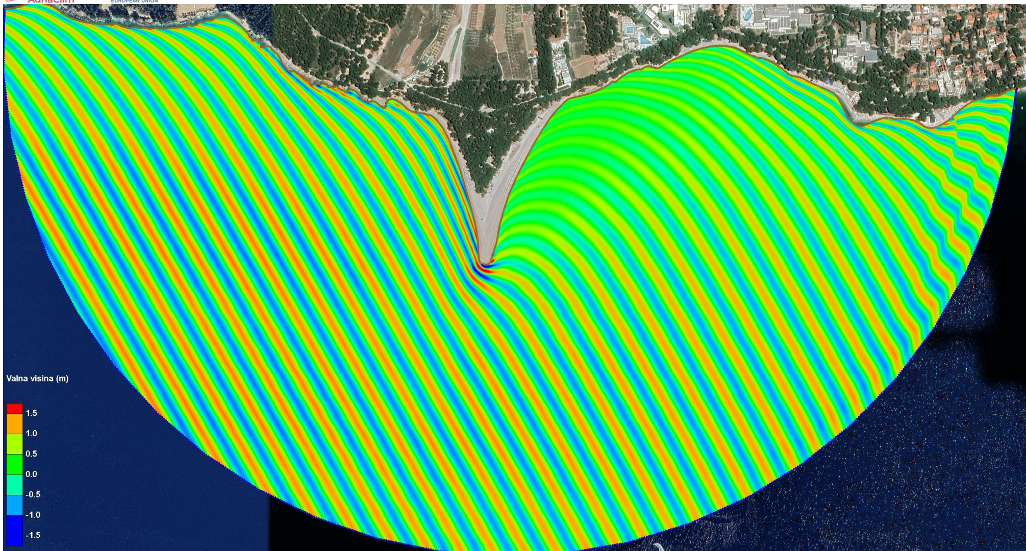
Figure 6.34 – Current wave outline for simulation for simulation A4 – existing state of Zlatni rat beach (Brač) with wave parameters from WSW direction (247.5°), 50-year return period ( H_s=2.63 m; T_p=6.61 s) and sea level corresponding to middle sea level (SRM)
