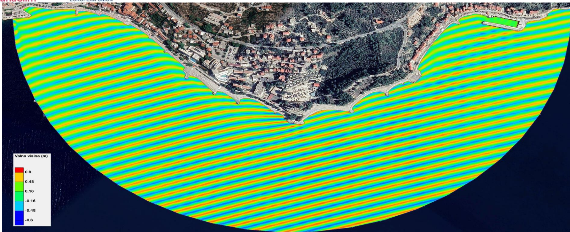
Figure 6.46 – Current wave outline for A12 simulation – existing state of Podgora beach (Makarska Riviera) with wave parameters from SW direction (225°), 50-year return period ( H_s=1.45 m; T_p=4.91 s) and sea level corresponding to middle sea level (SRM)
