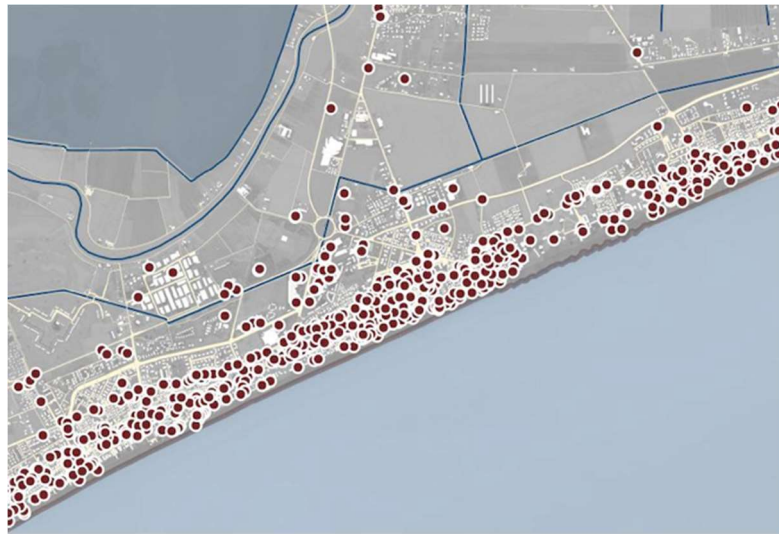
Figure 18. Fragment of cartography of the Municipality of Jesolo showing the points of interest extracted by mining from OpenStreet Map. In this image, it is possible to appreciate the density of economic activities and services that have been considered to estimate the density of elements exposed to Multi-Risk (MR)
