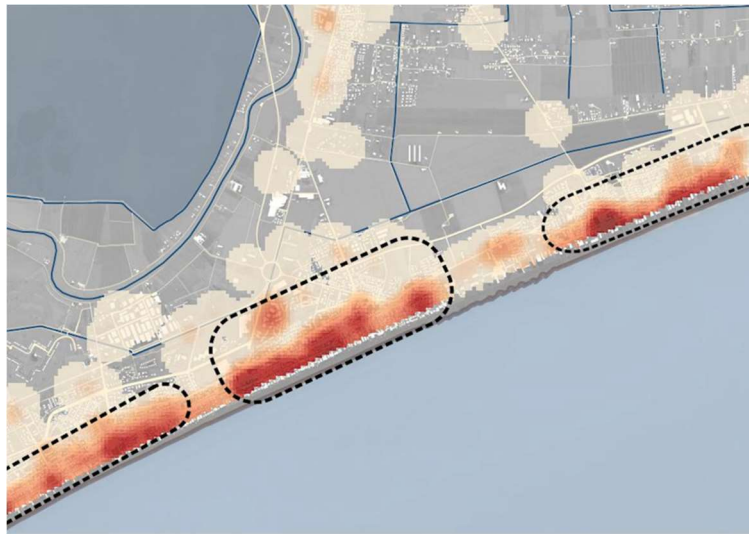
Figure 19. Extract of cartography containing the density estimate of the OSM points, conducted on the Municipality of Jesolo using kernel density algorithms, to spatially identify the contexts richest in elements potentially exposed to the MR (which is shown in the next image, Figure 4). This image represents one of the variables with which the multiple risk factor will then be calculated and supports the structuring of the adaptation process by orienting it towards targeted planning of those that may represent stakeholders for the initiation of policies and practices in response to the changing climate to be included in urban governance.
