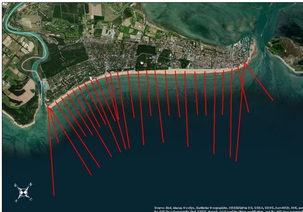
Figure 20. Planimetry of topo-bathymetric profiles of the Lignano coast (courtesy of Coastal Group).
