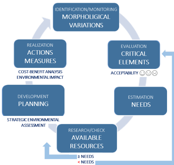
Figure 12. Proposed scheme for a correct approach to coastal erosion assessment and management (from MATTM-Regioni 2018, modified).
