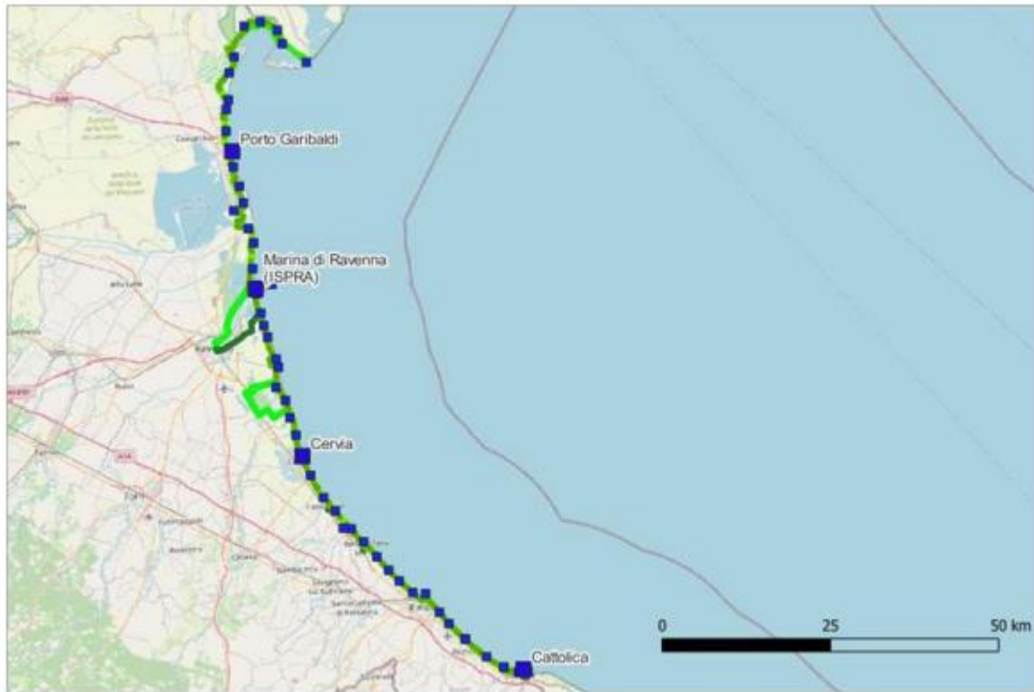
Figure 4.4: benchmarks of the RGC (Rete Geodetica Costiera, Coastal Geodetic Network) along the Emilia-Romagna coasts
