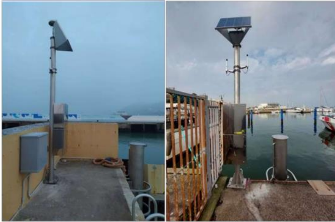
Figure 4.6: new tide gauge with co-located GNSS permanent station of Cattolica (left) and Cervia (right)
