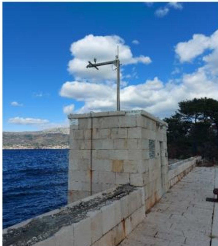
Fig. 2.8.4. Meteo - oceanographic station Punta Jurana with tide gauge housing.
