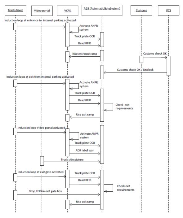
Diagram 9: Exit procedure from harbour area - sequence diagram
