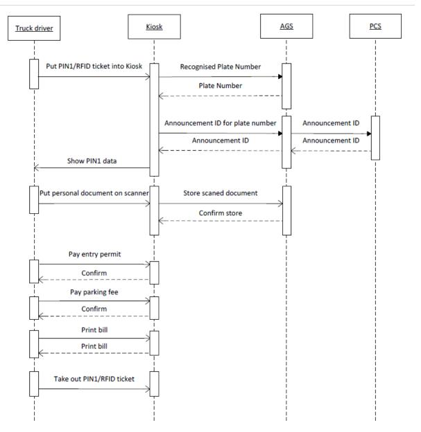
Diagram 4: Identifying driver, vehicle and bill procedures - sequence diagram
