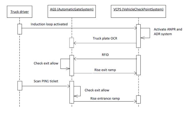
Diagram 5: Exit procedure from external parking lots - sequence diagram
