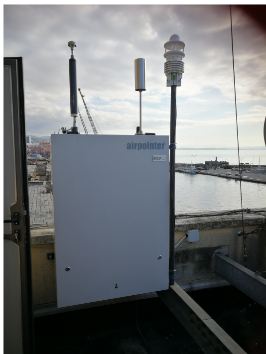
Figure 12. Compact monitoring system (Air Pointer, Recordum, Austria) used to monitor NO 2 , PM 10 and O 3 in the harbour area
