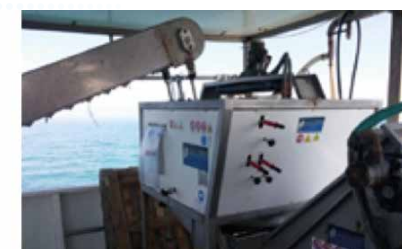
Fig.29B Mussels declumper machine
