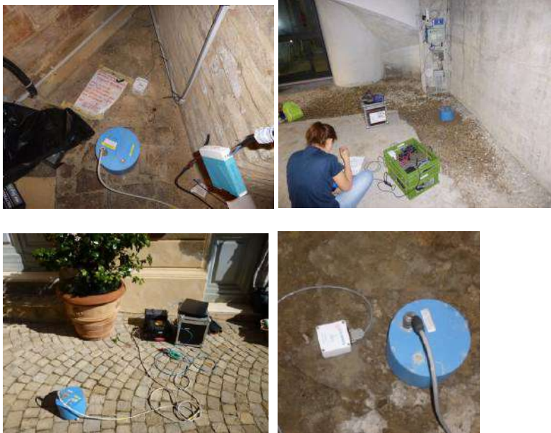
Fig. 2 examples of SPBs – temporary seismic stations measurements
