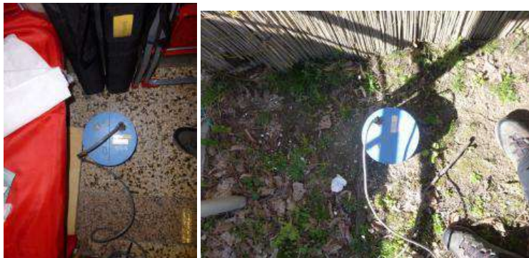
Fig. 1 examples of SPBs – permanent seismic stations implementation
